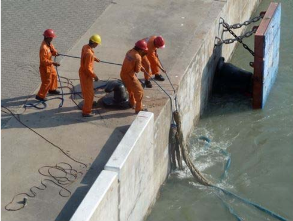
Tying up to the wharf. The ball is thrown from the ship with the lead line attached; then people (or vehicles) drag the heavy lines ashore.
